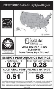
This window is Energy Star qualified in North, North-Central, & South-Central zones. Upgrade of SOLAR LOW-E qualifies window in South zone and provides: U-factor: 0.26, SHGC: 0.20, Visible Transmittance: 0.46
