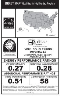
This window is Energy Star qualified in North, North-Central, & South-Central zones. Upgrade of SOLAR LOW-E qualifies window in South zone and provides: U-factor: 0.27, SHGC: 0.20, Visible Transmittance: 0.46
