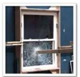
5300 AIP Windows carry a DP-45 rating in accordance with the American Architectural Manufacturers Association's 101 standard for air, water and structural wind load testing.
