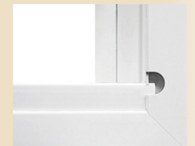
Tight, mortised-cut, double-wall sill dam extends inside the jamb, increasing durability and eliminating an open seam joint.
